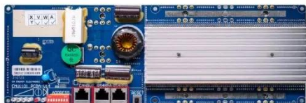
RS485 Communication between battery and inverters Band rate:9600bps RS485 Interface Communication between parallel packs of BMS and PC Band rate:9600bps
